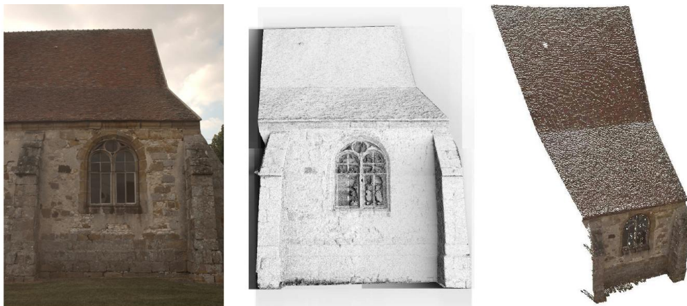
Figure 3: The multi-stereo image matching method: the master image (left), the matching result (in term of depth map) in the last pyramidal step (center) and the generated colored point cloud (right).
